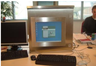
Fig. 2-5 : Enclosure of Control Touch Panel (Note: Contents of Enclosure are Expert Remote I/O module and Expert Embedded Board and Power Supply and Touch Screen)
