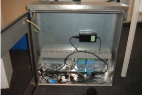
Fig. 2-1: Expert Remote I/O module and Expert Embedded Board and Power Supply and Wire Connection into Enclosure of Control Panel (Note: Embedded Board on back side of Wall Mount)
