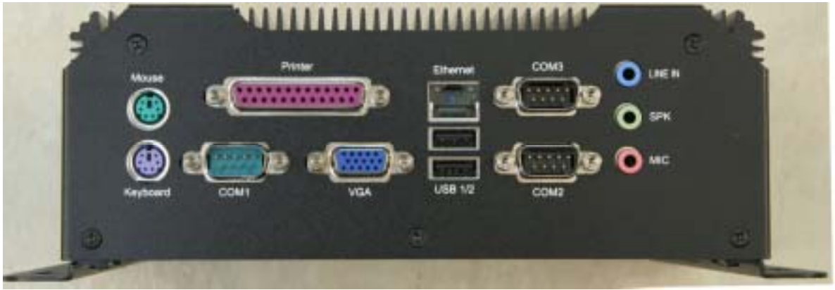
Figure 1.3: Rear View of EX-92630
